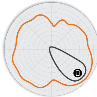
Figure 4. R550 2.4GHz Elevation Antenna Patterns
