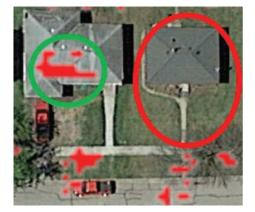
**Identify** determines green circled home on the left has coverage for desired install height above roof and red circle home on the right does not. Location and addressing information is provided for the home on the left and all similar buildings.
