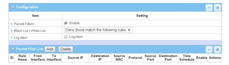
"Packet Filter" function can let you define some filtering rules for incoming and outgoing packets. So the gateway can control what packets are allowed or blocked to pass through it. A packet filter rule should indicate from and to which interface the packet enters and leaves the gateway, the source and destination IP addresses, and destination service port type and port number. In addition, the time schedule to which the rule will be active.
