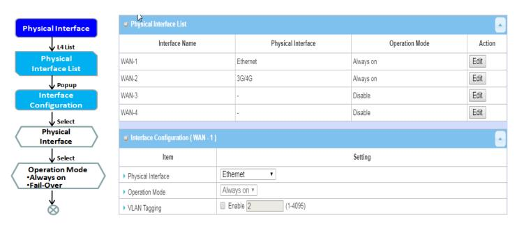
M2M gateways are usually equipped with various WAN interfacess to support different WAN connection scenario for requirement. You can configure the WAN interface one by one to get proper internet connection setup. Refer to the product specification for the available WAN interfaces in the product you purchased.
