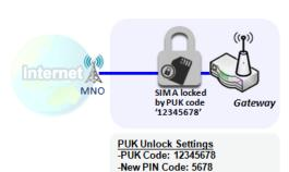
If you entered incorrect PIN code at configuration page for 3G/4G-1 WAN over three times, and then it will cause SIM card to be locked by PUK code. Then you have to call service number to get a PUK code to unlock SIM card. In the diagram, the PUK code is "12345678" and new PIN code is "5678".
