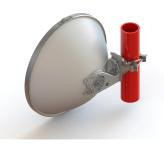
0.6 m | 2 ft ValuLine® High Performance Low Profile Antenna, single-polarized, 21.200–23.600 GHz, PBR220 flange, white antenna, composite broadband gray radome without flash, compact pack—one-piece reflector
