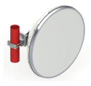
0.9m | 3 ft ValuLine® High Performance Low Profile Antenna, single-polarized, 21.200–23.600 GHz, PBR220 flange, white antenna, composite broadband gray radome without flash, standard pack—one-piece reflector
