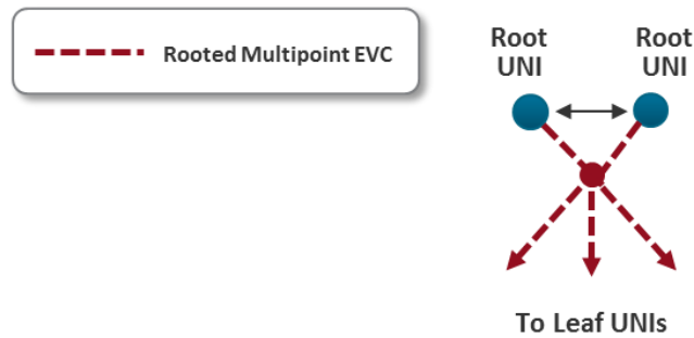
Figure 34 E-Tree Service Type Using Multiple Roots
